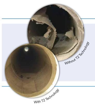
Chewout occurs when a core can't transmit the winding torque generated in a converting operation. This causes slippage of the chuck in the core, and ultimately leads to a core failure, and loss of web tension control.
